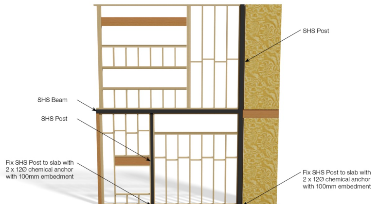
Images above and below show a typical 90x90 SHS steel wind beam and column that were installed to keep the wind beam size down when timber was not adequate.
