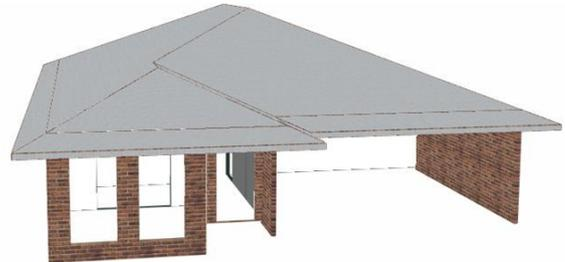
Fig 3 – Front facade of a house with large openings and a few 'brace-able' walls
