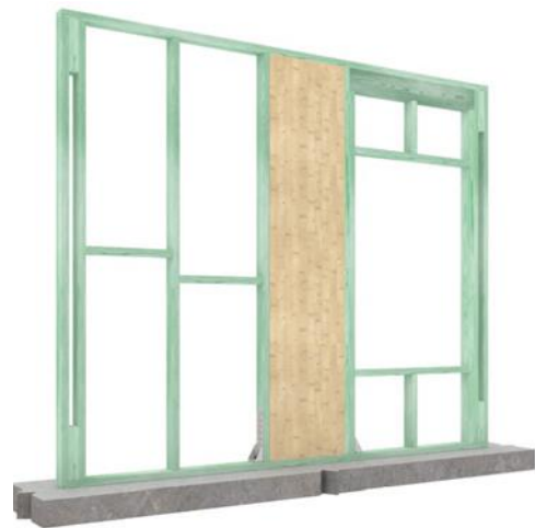
Figure 3: Example of a solid glulam bracing method.
