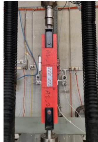
Pryda nailplate testing (load & plate orientation parallel to grain) for LVL
