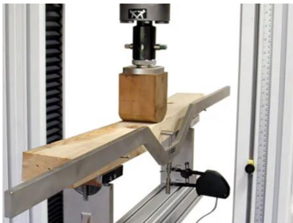
Source: Instron's bend test fixtures (3-point bending)
