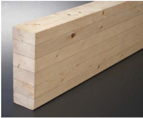
Fig. 2 – Typical Glulam section manufactured from softwood raw material.
