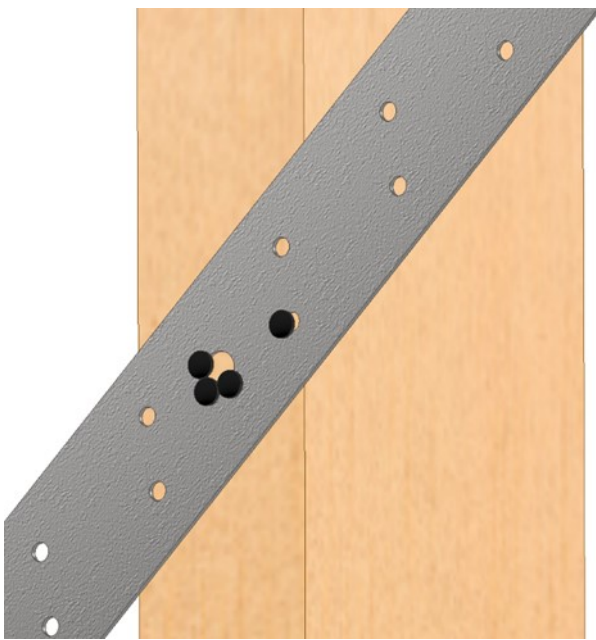
Figure 2: Poor installation. Nails have been installed too closely together and too close to the precut holes. The right-hand nail does not meet minimum edge distance requirements.
