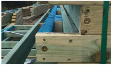
On this front, factory processes also provide the answer, ensuring the right screw goes in the right place, every time, at every connection point. Pryda offers truss and frame manufacturers a factory-fixed screw for the job.
