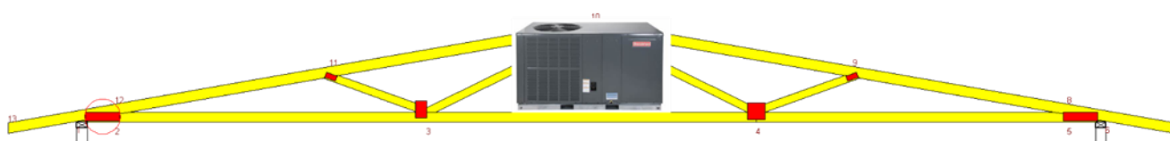
Figure 2: A low pitch truss which will create conflicts with housing the AC unit in the roof space
